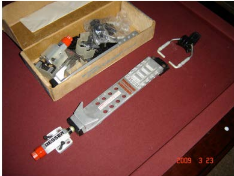
FIG. J. Besser design from later 1970s, allowing for release vertically and laterally at toe and heel.
